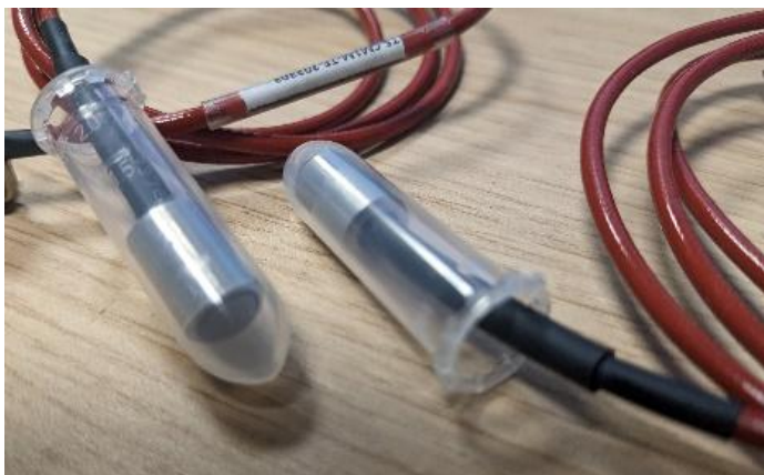
Fig. 1 Example of a DHF Series sensor: total heat flux with smooth-body interface.
