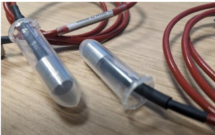
Figure 1 DHF heat flux sensors in their protective housing. Their thin sensitive film makes them very reactive, but must be carefully handled
